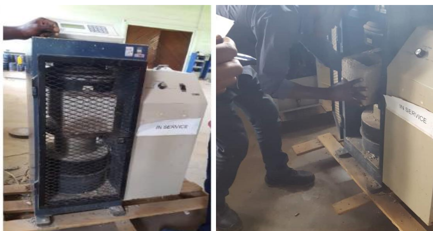
Figure 7. Compressive strength testing machine and testing procedure
