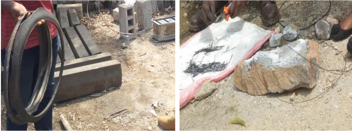
Figure 2. Wires extrusion from cut tyres
