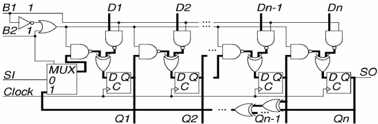
**Figure 2.2.** Multiple Input Signature Register
